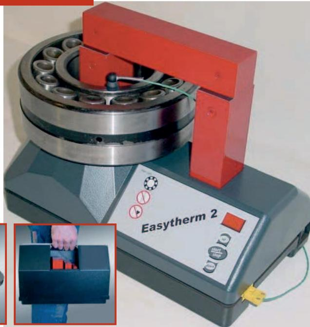
The Easy therm 2.0 is a small powerful microprocessor controlled induction heater for heating of small sized components including bearings up to 40 kg!! It is easy to use and portable, complete with a robust case, ideal to use on location.
