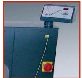
The Easy therm 100.0 is a robust powerful 400 Volt stationary microprocessor controlled induction heater, to be used for the professional mounting of heavy parts including bearings, typically used in maintenance shops and production areas, for instance paper-mills and steel-mills. With easy to fit lift installation and rail system for the parts, the Easy therm 100.0 can be assembled to an ergonomic production machine. (see optional parts)
