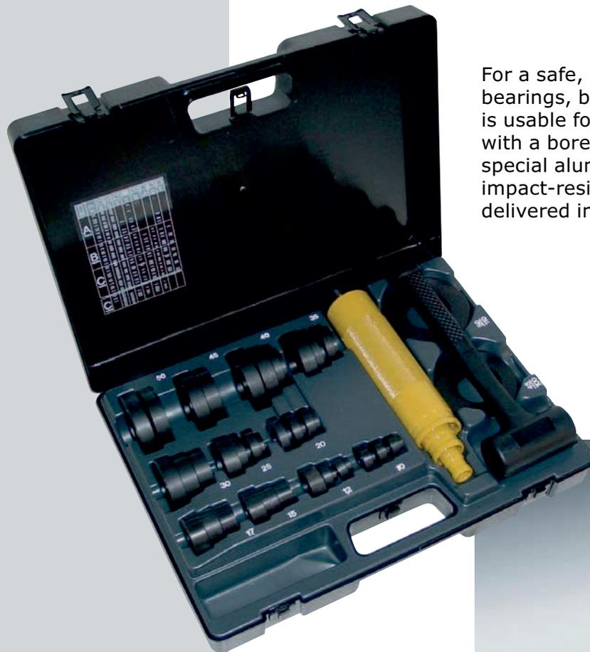
For a safe, precise and quick mechanical mounting of bearings, bushings, sealing rings and pulleys. This set is usable for fitting more than 230 sizes of bearings with a bore from 10 to 50mm. The set consist of three special aluminium impact sleeves, 33 synthetic impact-resistant collets and a dead blow hammer, delivered in a robust plastic case.
